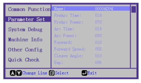
Press "▲"" ▼" to select, press the to enter the menu needed to change, press the "▲"" ▼" to change the Parameters, then press to save the results . When the changing finished, press to exit.
