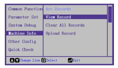
Enter "Arc times" menu by pressing ■■ and check arc records by pressing "◄", "▶" The machine can store 6000 times splicing arc records.
