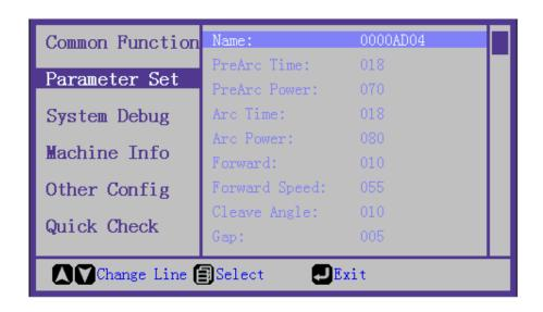
Press the "▲""▼" to select, press the to enter the menu need to be changed, press "▲""▼" change the detailed Parameters, then press the to save the result. When changing finished, press the Exit.
