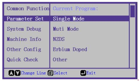
Press the "▲" "V" choose the Procedure Number you need to operate or change, press the Procedure you want(the red is the current Procedure operating). If need to change the Procedure Parameters, please repress to enter the Procedure to change the detailed Parameters (DEFAULT is Factory settings, cannot be changed)
