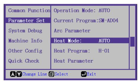
Press the to enter the "heat program" menu, press \( \Lambda \)" \( \nabla \)" to choose the working mode "Auto" or "Manual". When the choosing finished, press to save the results. When changing finished, press to exit.
